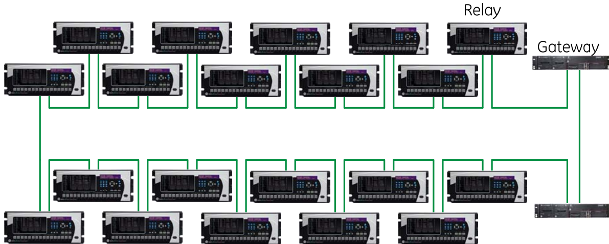
Figure 17: HSR network for transmission substation
