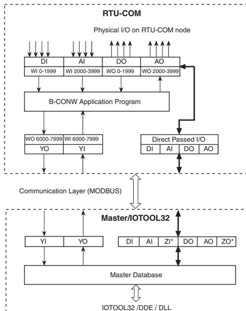
\*Zi/ZO is gateway I/O - not used in standard RTU8.
