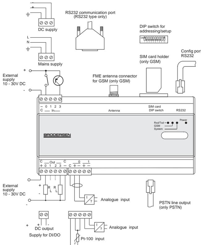
See the installation manual enclosed with the module, for more wiring details.
