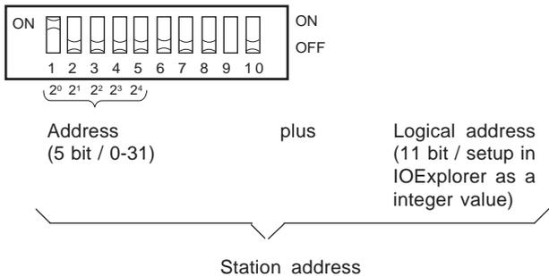
The Modbus address (physical address) is set to address 1 (independent of the switch) when modem control is enabled.
