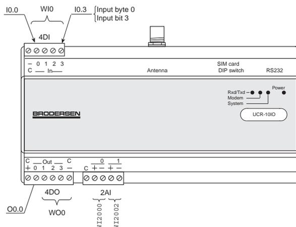
**RTU-COM / Compact outstation with built-in modem**
